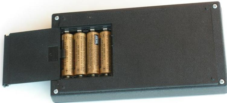
The batteries should be replaced when required by conditions described in section 1.3 above. Be careful to observe the positive and negative polarity
