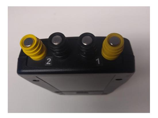
CAUTION: The pulses applied to these terminals may be as high as 316 volts when the output is fired. This will result in a painful, and possibly lethal, electric shock to a person touching these terminals or the connected cables at the moment they are fired. BE CAREFUL! Do not touch them unless the module power has been off for at least 45 seconds.
