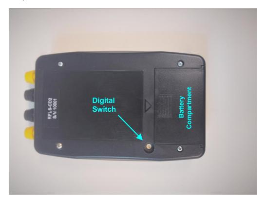
The battery should be replaced when required by conditions described in section 1.1 above. Be careful to observe the positive and negative polarity markings in the battery compartment when installing the battery. In order to prevent damage to the module from battery leakage, the battery should be removed before storing the module for long periods of time. To prevent battery depletion and resulting leakage, be sure the power is turned off when the module is not being used.
