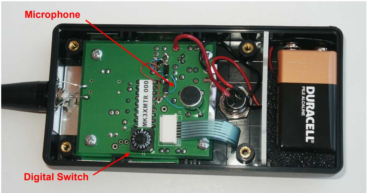
(Transmitter with rear cover removed)
